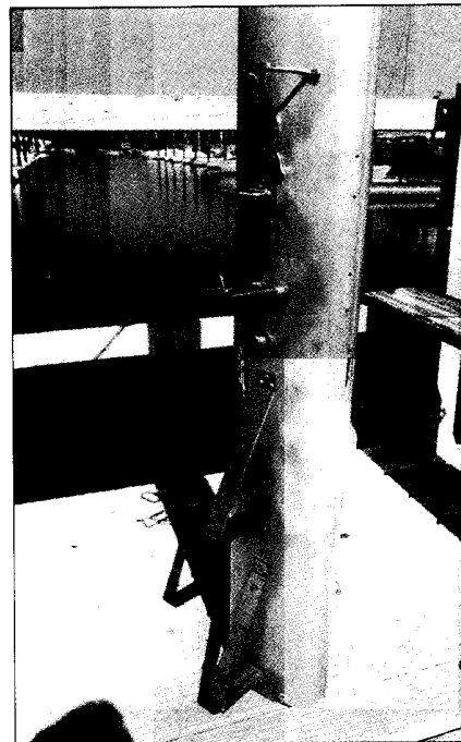
Above: Shown here are three views of the nine mast steps discussed. In each view, the steps are, from the bottom left up, The stainless West Marine triangular step; the ABI triangle; the Fastep, fashioned of stainless rod; the ABI folding step that works better on a transom, and the little Ronstan, an old design that is very popular. On the right side of the mast are, from the bottom up, the flattened aluminum tube sold by Defender; the Pace-Edwards extruded aluminum step; the folding Almag Mast Walker, and ABI's very similar cast aluminum version.
