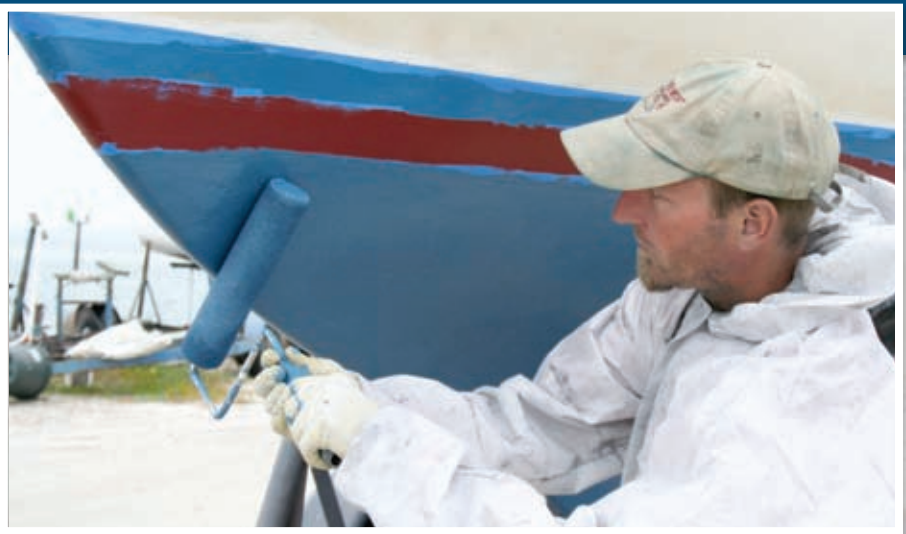
After nearly a yearlong review, PS testers decided the only thing cayenne pepper in bottom paint increases is drag. Mixed with Interlux Bottomkote, it had no impact on antifouling protection on this Cape Dory 25.
