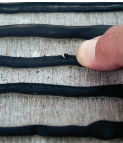
BoatLIFE Teak Deck Sealant performed in the middle of the pack. After two years, the test beads had dried out and were cracking.
