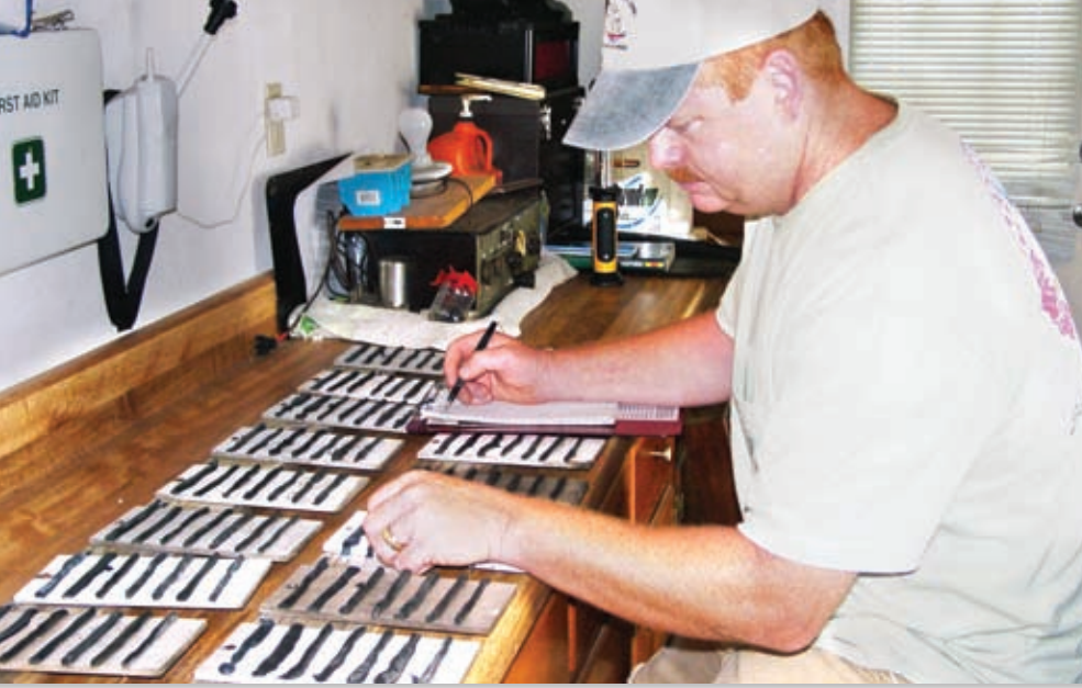
Beads of each test caulk were applied to more than a dozen wood panels, which were mounted outside and exposed to various chemicals regularly.
