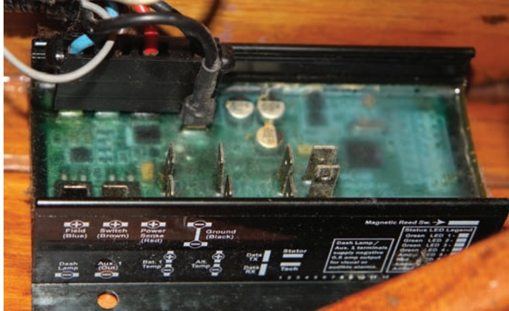
The multi-stage Xantrex XAR alternator regulator (above) was set to match the charging specs for the Trojan T105. Victron’s BMV-501 (right) kept accurate track of the battery system’s health.
