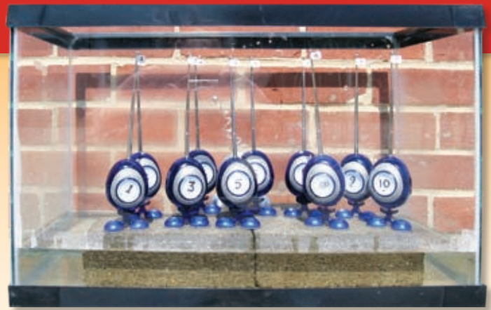
These cheap radios were sprayed with electrical protectants and then left to sweat it out in the humid atmosphere of an aquarium containing sea water.
