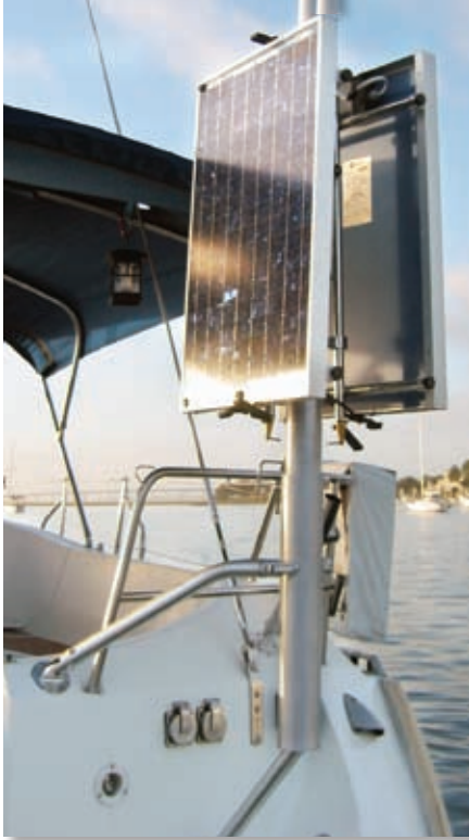
Solar Stik allows the panels to fold down and lock securely into place.
