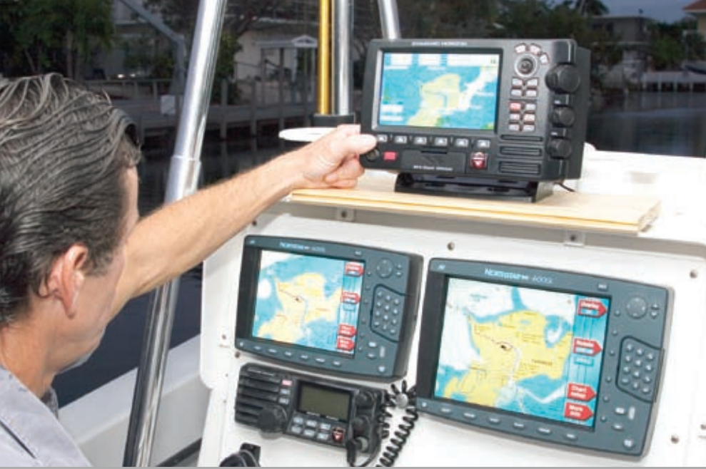
The Standard Horizon CPV350 (top) is a marine VHF radio and chartplotter with a hailer and foghorn. It also has sounder capabilities.
