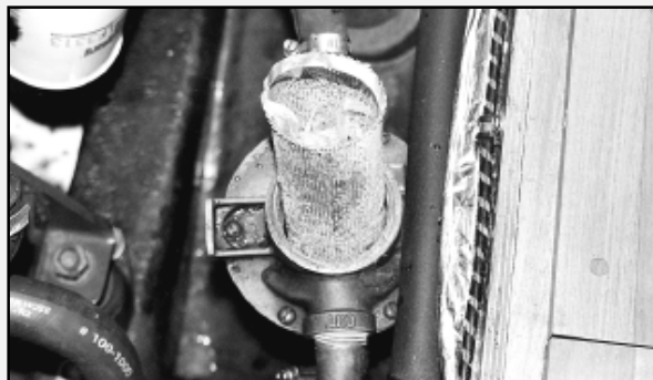
We were surprised to find our raw water strainer completely clogged with a shredded plastic bag.
