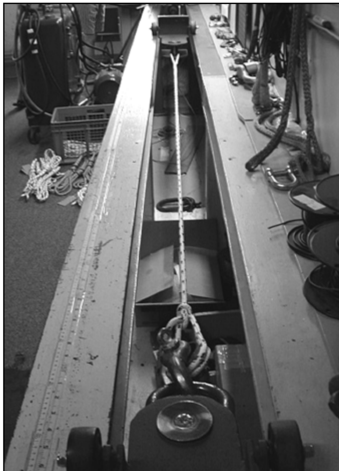
Left: The hydraulic pulling rack at Aramid Rigging in Portsmouth, Rhode Island. Aramid's professionals set up many sample lines with eye splices at the stationary ends. The working (pulled) ends included eye splices, bowlines with two round turns, anchor bends, constrictor knots, and clove hitches. Knot-induced weakness notwithstanding, it soon became clear that these common high-techs are just too slippery to hold standard hitches at any reasonable pressure—so buntline hitches were added to many, just to keep them in place to be broken. Below: Aramid's production manager Brian Fisher gathers read-outs after putting the screws to the ropes.
