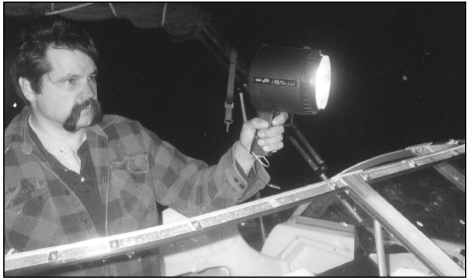
The lights were taken out on the Powerboat Reports test boat and shined on a green navigational buoy from about 900 feet away. We noted strength of illumination, and how much scatter each light generated.
