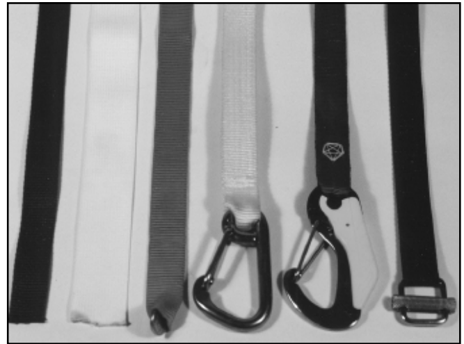
From left to right are six samples of webbing. Purchased from West Marine and fine for light duty are the 1" dark-colored piece and the 1-1/2" white piece of flat webbing. Third from the left, with a nickel in the end to show its construction, is a good piece of tubular webbing. Shown securely sewed to a Wichard snap hook is an even better piece of white tubular webbing made up as a life harness tether; note the generous and excellent sewing. Second from the right is a piece of flat webbing glued and sewn, (in a questionable way), to the relatively new Wichard double-action hook. On the far right is a piece of thin, very cheap webbing glued (not even sewn) to a sliding bar buckle. This was taken from an old child's backpack. The terminal here is much sturdier than the webbing; today it would be replaced by a plastic clip.
