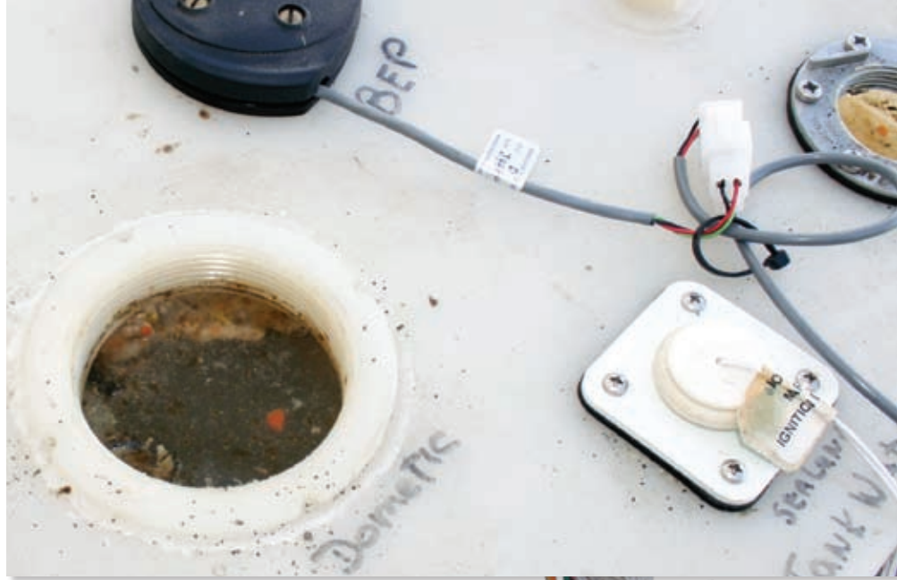
The fake effluent developed into a smelly, dark liquid after nine months in the test tank.
