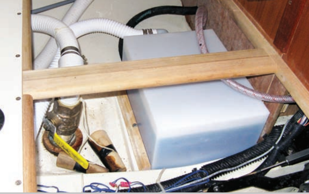
Midnight Rider's do-it-yourself freshwater flusher cuts down on head odors.
