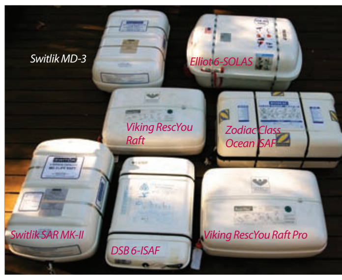
Seven of the eight rafts PS tested came in canisters. Their weights ranged from 84 pounds for the DSB ISAF (front, center) to 167 pounds for the Elliot SOLAS (back, right).
