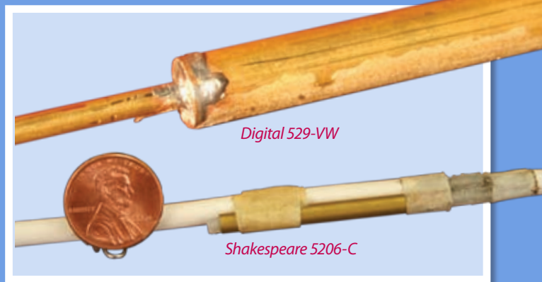
Testers found that the radiating element of the $36 Shakespeare 5206-C is significantly thinner than that of the $149 Digital 529-VW.
