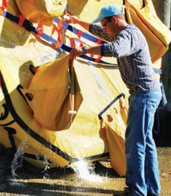
Winslow's retractable ballast bags let the raft be sailed downwind.
