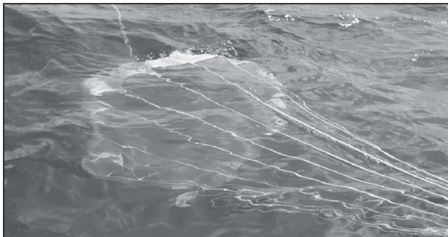
The Fiorentino FPA-9, above, fully deployed with its 16 shroud lines showing prominently. The theory here is that more shroud lines make the canopy less prone to inversion when the waves really kick up. This sea anchor is rated by the company for boats under 40 feet and under 20,000 lbs.
