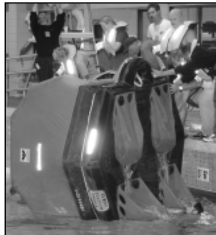
The Viking was turned upside down and quickly righted itself. Note the water-ballast bags.
