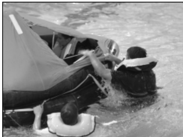
Boarding a liferaft in a PFD is no easy matter in a well-lighted wave pool, even for a person in good shape. Design of boarding aids is critical.
