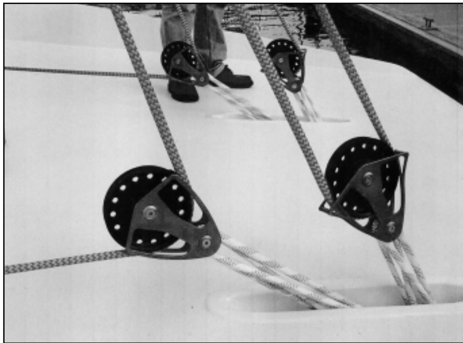
Doubled (or 'basketed') Yale Loups restrain the blocks for runners and checkstays on a modern racer. The blocks have to be disassembled to accept the loops. If such a loop is to live in a padeye, it has to be made in place.
