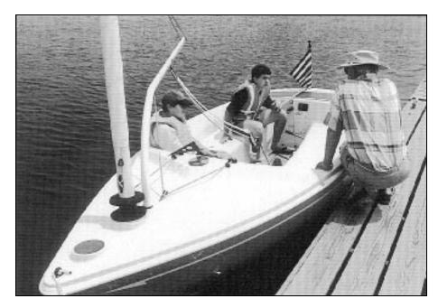
With Garry Hoyt, the EXPO's developer, standing by, our two teenaged test pilots look over the boat's layout and controls. Note the wind vane mounted on the deck forward of the cockpit, the simple engine control handle and the big solar panel on the stern deck.
