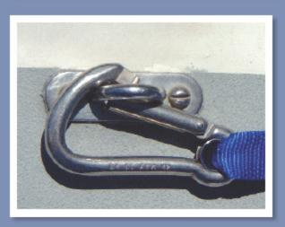
The International Sailing Federation (ISAF) Regulations Governing Offshore and Oceanic Equipment and Preparation, Rule 5.02.1, warns, "It is possible for a plain snap hook to disengage from a U-bolt, if the hook is rotated under load at right angles to the axis of the U-bolt. For this reason the use of snap hooks with positive locking devices is strongly recommended."
