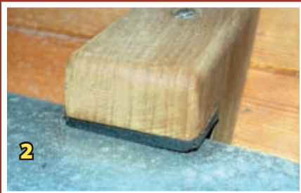
1. Stainless-steel bushings insulate copper-alloy (brass, bronze) fittings from tank. 2. Non-hydroscopic material (preferably adhered to tank itself) isolates tank from wood. 3. Install inspection plates into every baffled chamber. 4. Leave at least a 1/4-inch air gap between bottom of tank and its shelf.
