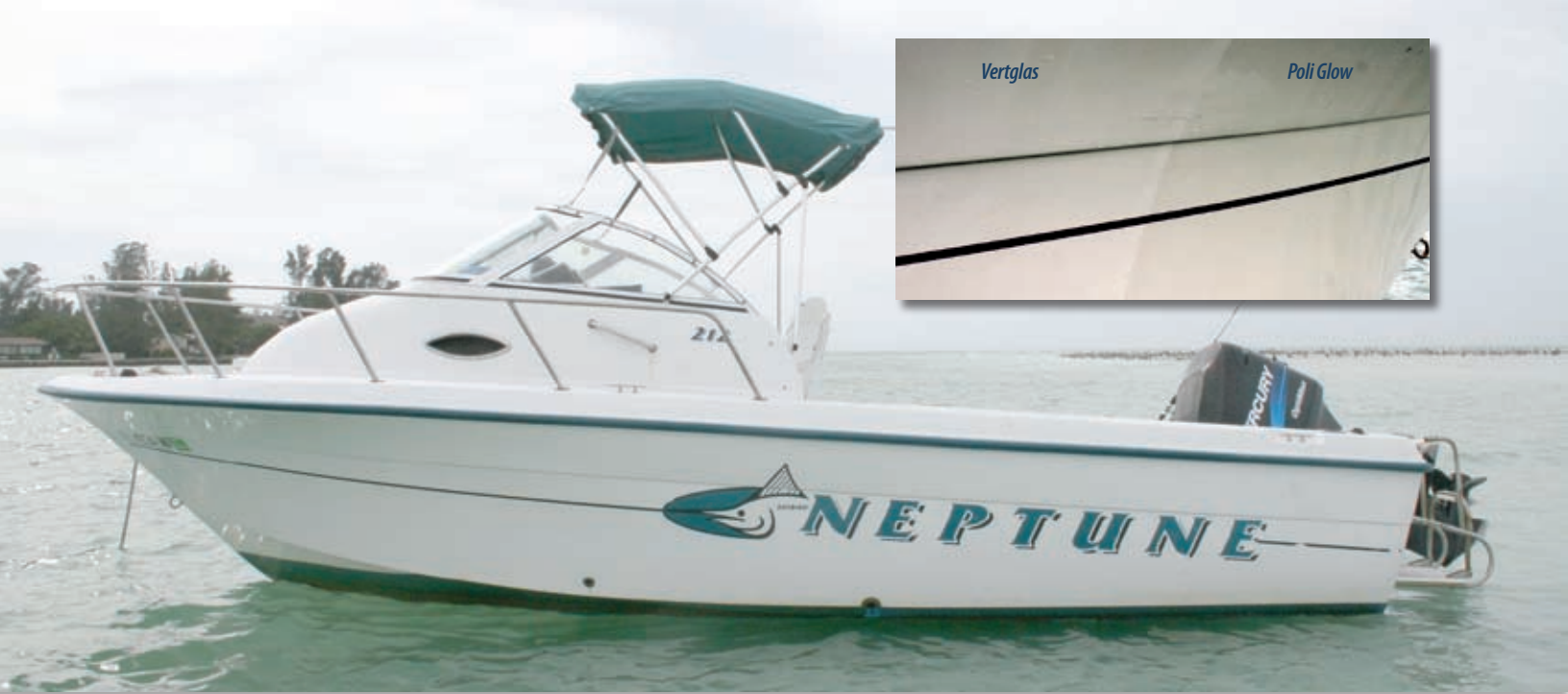
In 2003, testers coated this boat's hull with three hull restorers: Poli Glow (bow), Vertglas (amidships), and New Glass 2 (aft and stern). Poli Glow's sheen (above) and water-beading action (inset right) are still visible on the boat's bow.
