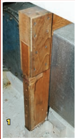
1. Direct contact between wood cribbing and the tank invites corrosion. 2. Stick-on foam insulation traps moisture. 3. Uncoated mild steel will corrode quickly. 4. Placing a tank where bilge water sits accelerates corrosion.
