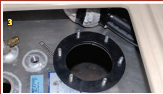
1. Stainless-steel bushings insulate copper-alloy (brass, bronze) fittings from tank. 2. Non-hydroscopic material (preferably adhered to tank itself) isolates tank from wood. 3. Install inspection plates into every baffled chamber. 4. Leave at least a 1/4-inch air gap between bottom of tank and its shelf.
