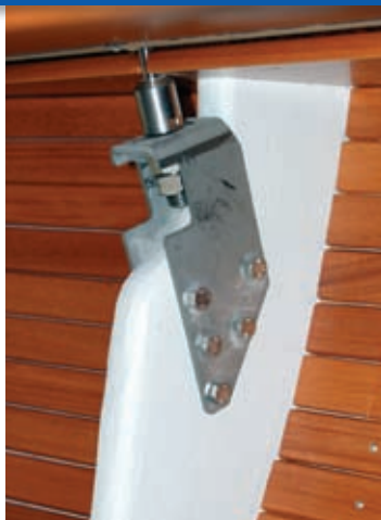
Inboard shroud chainplates are readily accessible for inspection.
