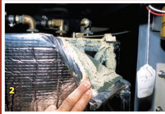
1. Direct contact between wood cribbing and the tank invites corrosion. 2. Stick-on foam insulation traps moisture. 3. Uncoated mild steel will corrode quickly. 4. Placing a tank where bilge water sits accelerates corrosion.
