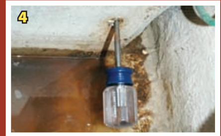
1. Direct contact between wood cribbing and the tank invites corrosion. 2. Stick-on foam insulation traps moisture. 3. Uncoated mild steel will corrode quickly. 4. Placing a tank where bilge water sits accelerates corrosion.
