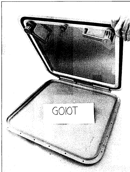
Above left: Goiot's Cristal hatch has a strong cast aluminum lid with a fair clear anodized finish. However, the frame base is an extrusion, rough anodized (in the European fashion) to give the impression that it is cast aluminum. Available in 16 sizes with several finishes, it has good dogging levers. The spring-assisted lid has an oddly-designed, adjustable-friction, burglar-proof hinge that is not pre-assembled, which makes the installation (with machine screws) somewhat difficult. Once installed, the hatch operates smoothly and securely. Above right: Hood's stainless steel hatch is a heavyweight. Made of extruded stainless that is finely finished on the outside but indifferently finished where it doesn't show, the hatch also suffers from some crude welding of the extrusion closures and the dogging plates. It has excellent, spring-loaded, adjustable dogs. The two support arms are well-made and have notch locks operated by clever spring-loaded twist knobs that help when opening and securing this heavy hatch. Very handsome, very rugged, very heavy to operate.
