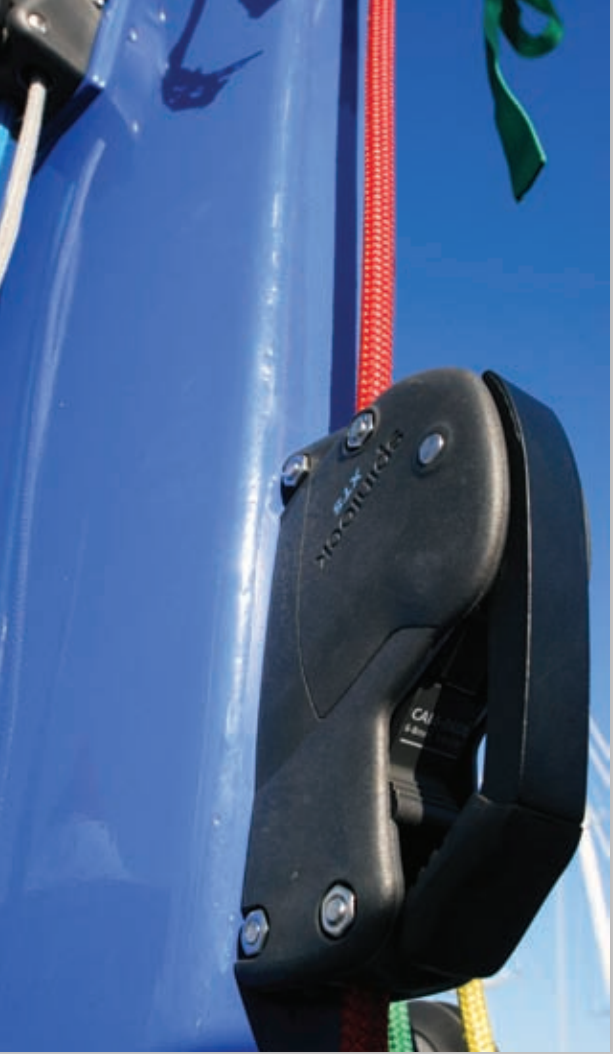
This mast-mounted Spinlock XTS reflects an effective use of a rope clutch. Boats that use spinnaker poles frequently might want to upgrade to an aluminum body.
