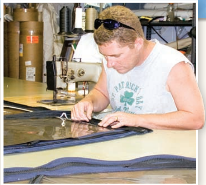
Eric Kolek of American Canvas in Sarasota, Fla., installs a zipper on a clear-vinyl window for an enclosure on a sportfishing boat.
