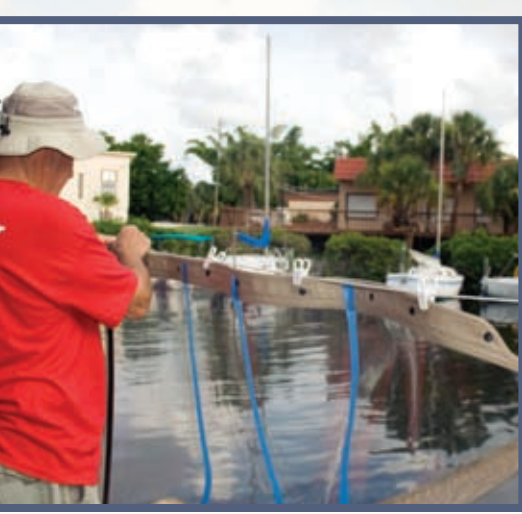
The clear-plastic cleaners/polishes test panel was left in the sun and salt air to weather for 30 days.
