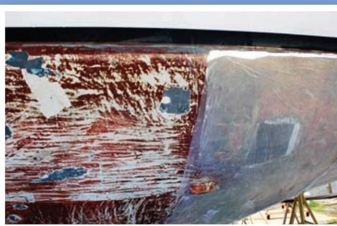
A 1-mil sheet of plastic was used to cover the Soy Strip to keep the chemicals from drying out. Peel Away recommends its own paper or regular butcher paper.
