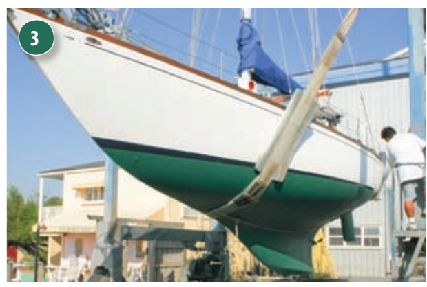
Breaking it down and building it up: The bottom 1. post haulout and pressure washing; 2. after two weeks of scraping and stripping; and 3. the final product after barrier coats and bottom paint are applied.
