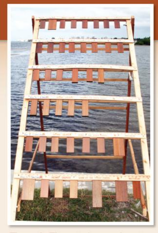
The rack: The exterior wood coatings that we're testing will all be mounted, and the rack will be left to weather South Florida's heat, humidity, rain, and occasional chill.
