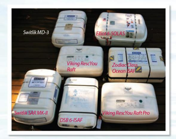
Seven of the eight rafts PS tested came in canisters. Their weights ranged from 84 pounds for the DSB ISAF (front, center) to 167 pounds for the Elliot SOLAS (back, right).
