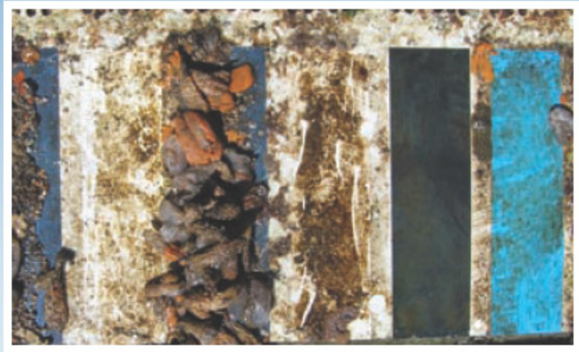
Several paints had lost their oomph after two years in Long Island Sound, allowing a lot of hard growth (above) and earning Poor ratings.
