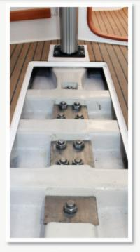
Keel bolts fasten through a large loadbearing plate recessed beneath the floors, part of a structural grid that absorbs sailing loads.
