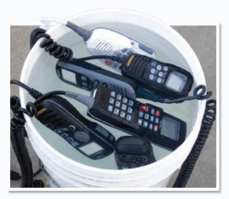
All six test mics were submerged for 30 minutes in fresh water and then operated to test their waterproofness. All passed the dunk test.
