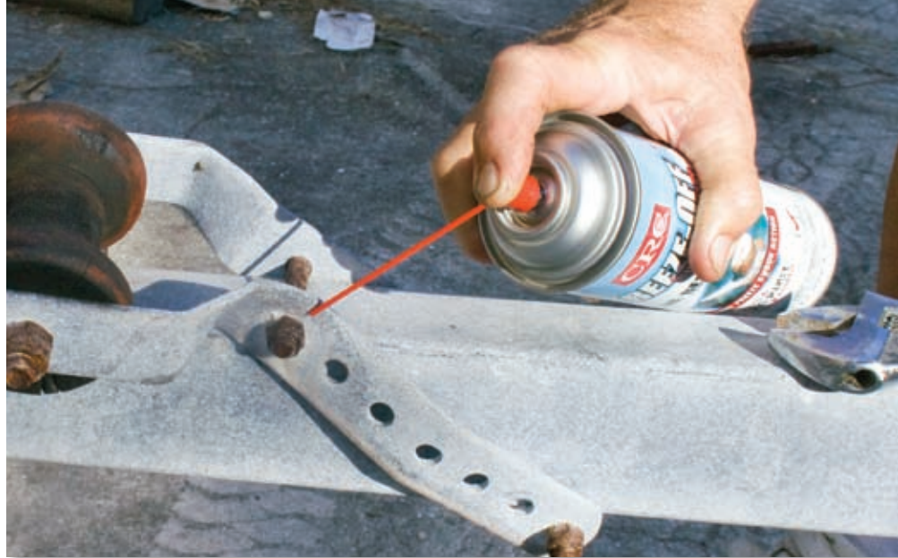
Frozen fasteners on a PS trailer sparked a test of four rust-busting penetrating sprays: CRC Freeze-Off (above), WD-40, Liquid Wrench, and PB Blaster.
