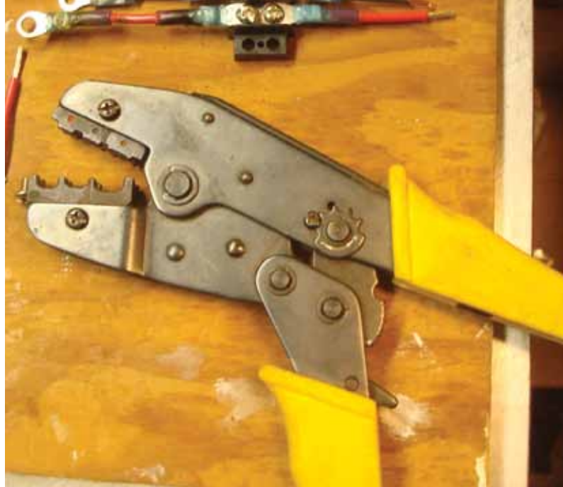
A good dual crimper with hardened removable dies can be bought at an electrical supply house for $40 to $70.
