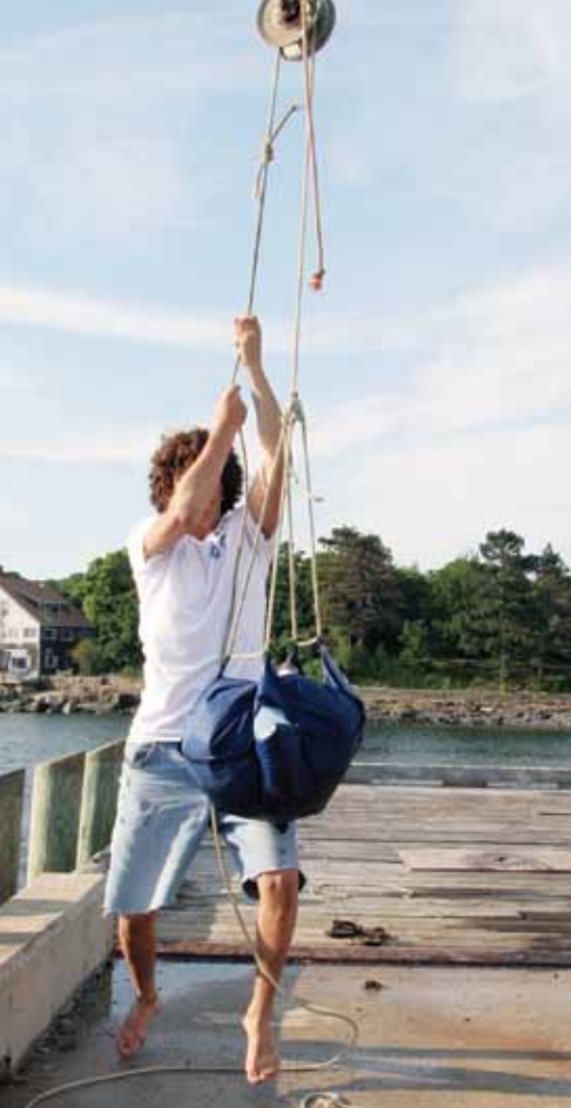
The Plastimo collapsible water tank undergoes a drop test.
