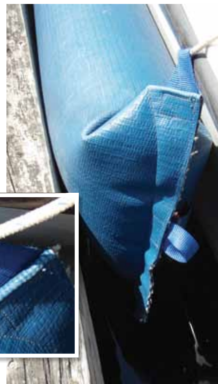
The Seoladair fender has been in steady use against a wooden dock and other boats, but it exhibits very little wear, even where it's hung from webbing loops.
