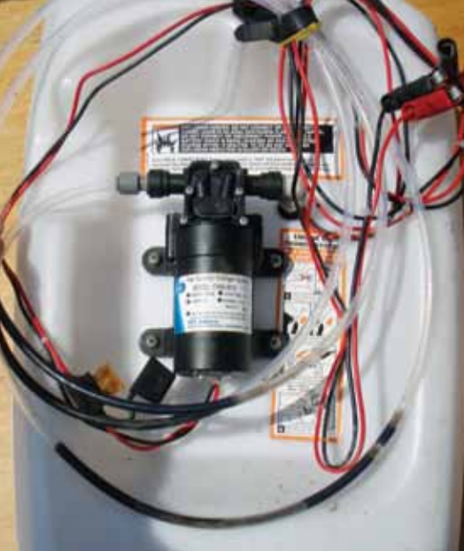
The Jabsco setup makes oil-changing quick and clean, but the unit is bulky and the suction tube is hard to clean.
