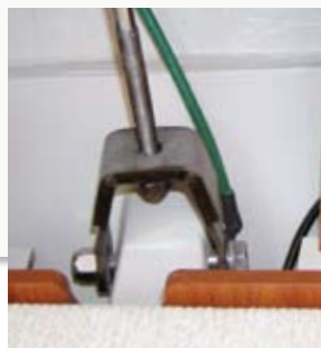
Tie-rods link the chainplates to U-shaped brackets that are bolted into the hull's structural grid.
