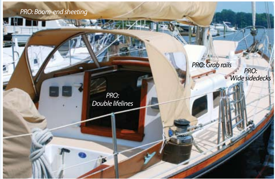
Solid construction practices and a sensible design make a well-equipped and maintained Pearson Rhodes 41 eminently capable of offshore sailing.
