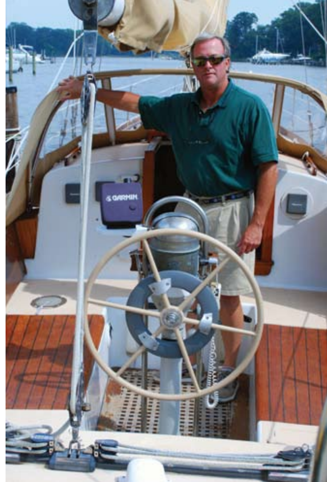
The Pearson 41, Lightfoot, owned by George Dunigan (above), is equipped with wheel steering. Phil Rhodes' original design called for a tiller.
