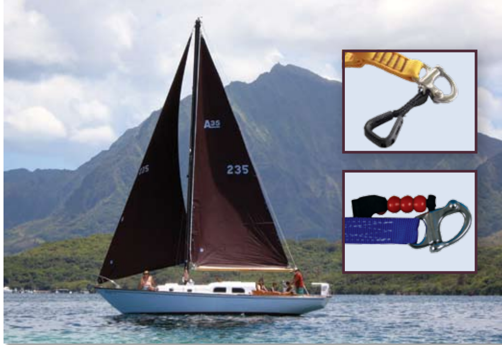
Reader Jack Durham, here aboard his Alberg 35, is retrofitting the pull cord on his new West Marine tether (top) with beads to resemble his older WM tether model (bottom).
