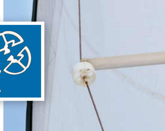
Several companies market shroud rollers to fit below spreaders. Practical Sailor is testing a set from Forespar made by Wave Marine Products (above left); the Sail Savers now come in blue.
