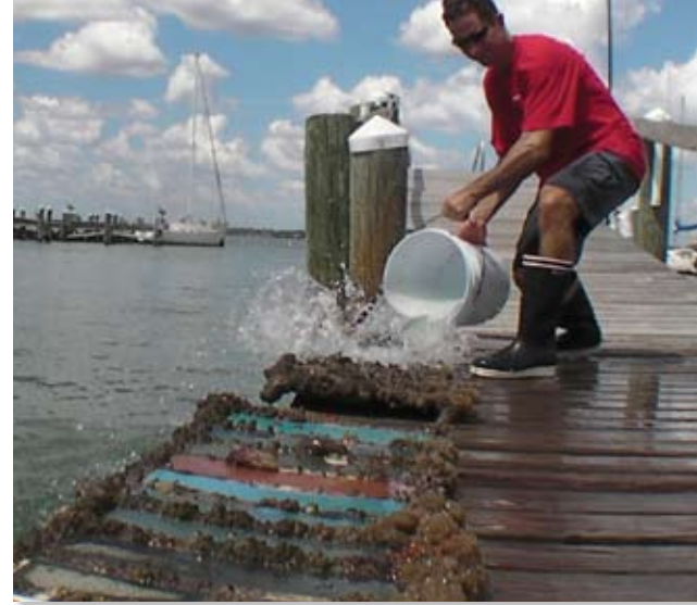
All but a few paints proved very effective at combatting hard growth for six months.
