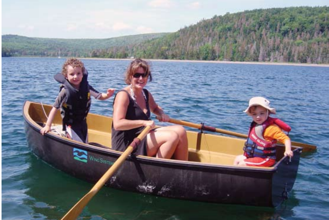
Lightly loaded, the Wing Dinghy presents very little wetted surface. It can carry over 1,200 pounds and still have 5 inches of freeboard.
