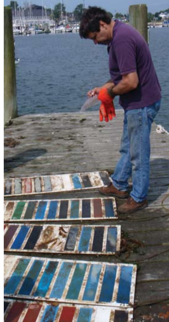
Paint test panels were pulled and rated in June. The above panels were immersed in a marina in Stamford, Conn.
