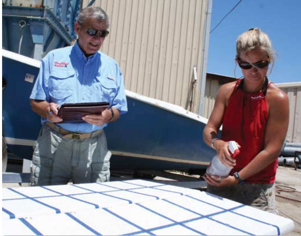
Testers compared each test product's ability to bead water on the fiberglass panels, in both horizontal and vertical positions.
