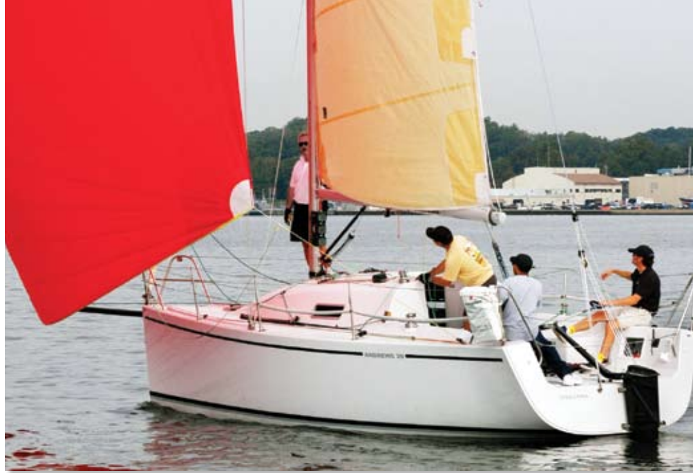
Comparing the Andrews 28 to one of the more nimble classic plastics of similar length reflects how advances in composite technology has allowed builders to drastically reduce hull weights. Despite carrying almost the same working sail area, the Andrews weighs in at less than half of the Pearson 30, one of the "faster" boats reviewed in our April 2008 issue that looked at 30-footers from the 1970s.
