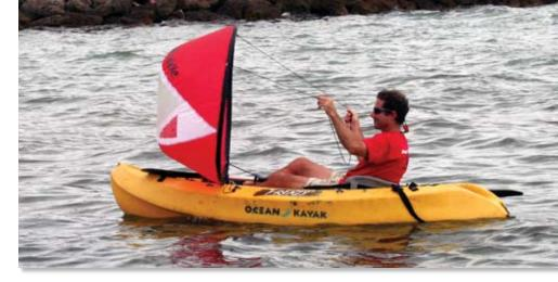
The WindPaddle is made of half-ounce rip-stop nylon and has a window that offers good visibility. The sail is controlled by thin, lightweight sheets attached to the sail's top.
