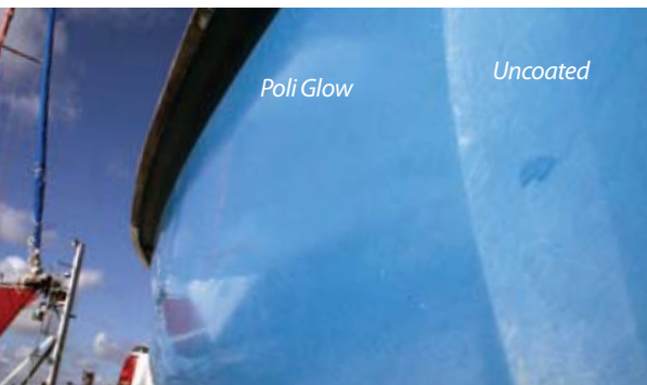
The Poli Glow-treated section of the hull reflects images of nearby boats at the Sarasota Sailing Squadron in Florida. The chalky area does not have any coating.
