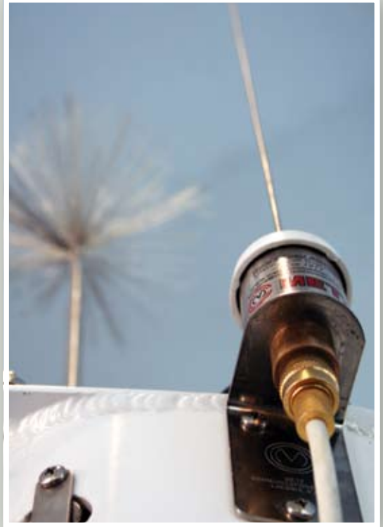
Mounting the VHF antenna on the mast and the AIS antenna on the stern rail will reduce possible interference.
