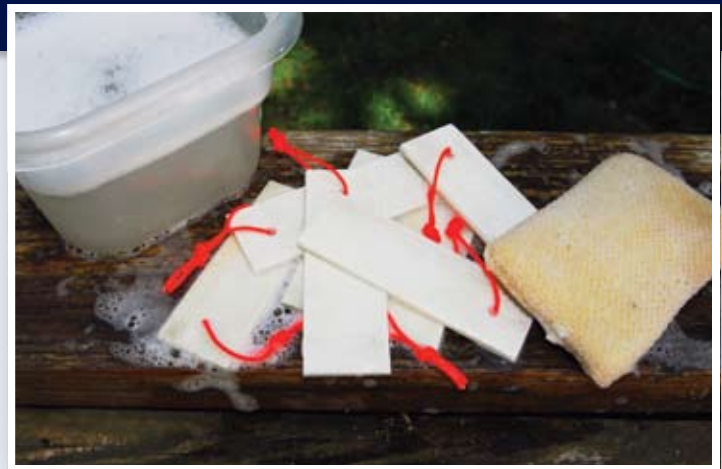
We prepped the test panels as we would any FRP surface we planned to use a sealant on, cleaning it well to erase any contaminants like wax, oil, or dirt and dust.
