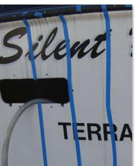
A blighted Morgan Out Island 41 was the test platform for our 2006 black-streak cleaners test. The streaks develop as polluted rainwater dries on the hull. The best remover we tested was made by Nautical Ease.
