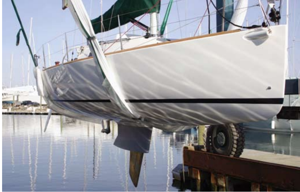
The J/95's bronze centerboard drops from a pocket in the lead-ballast keel. The pin assembly is held in place with 10 bolts and can be removed for inspection.
