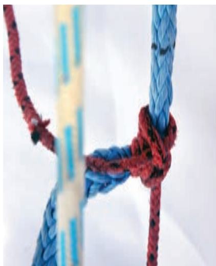
..... The regular rolling hitch (photo at far left) started at the blue tape and slipped under minimal tension. This hitch slipped on every material during testing except the large-diameter Dacron double braid. The modified rolling hitch (photo at immediate left) slipped on the Spectra single braid under moderate tension; the knot started at the black mark.
