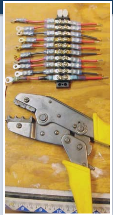
Used properly, a good-quality ratchet-style crimper offers consistent crimps that resist corrosion.
