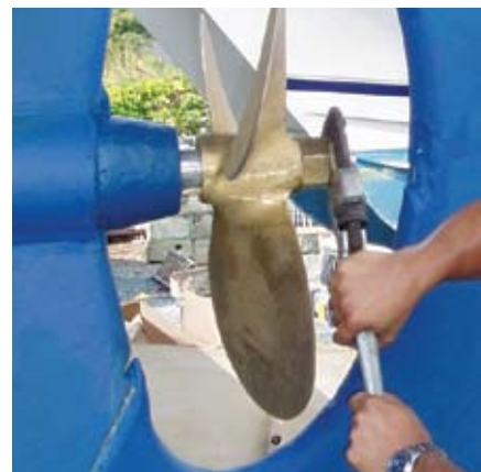
This photo shows the WRONG way to install a prop. The setup should be: prop, thin nut, large nut.
