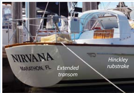
Nirvana, the 1974 H49 we tested, sports a 4-foot transom extension (photo below right). Compare her stern to that of Circe, the H49 pictured on page 8.
