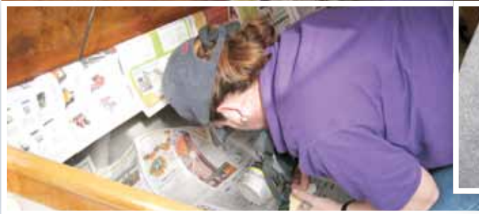
The crew protects adjacent surfaces with newspaper before spraying the adhesive for the carpet. Thin, flexible carpeting replaced the wornout vinyl headliner. Peregrine, a Beneteau First 235, sits on her mooring at Lake Jacomo, Mo.
