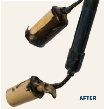
..... The rubber coating on the Groco float sensors we tested suffered a chemical breakdown. The maker said the problem was not common and would be covered in the warranty.
