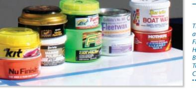
The 10 test paste waxes were applied to a fiberglass panel and left out in the Florida sun and rain for six months. From left, top row: Kit, Meguiar's Premium, Turtle Wax Super Hard Shell, Collinite No. 885, and Star brite Boat Wax. Bottom row: Nu-Finish, Star brite Marine Polish with PTFE, Turtle Wax F21, 3M Marine Ultra Performance, and Mother's Carnauba Cleaner Wax.
