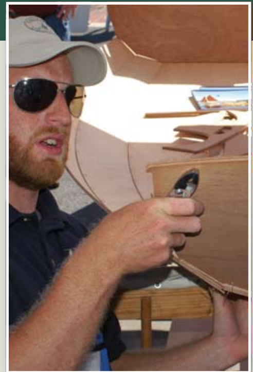
Precut strakes on a Chesapeake Light Craft are stitched together for bonding.
