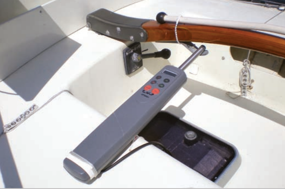
At sea, tester Skip Allan used high-strength tape to secure a lanyard to the Raymarine ST1000 Plus. He also covered the unit with a custom-made case. The cockpit hatch allowed him to make steering adjustments without leaving his bunk.
