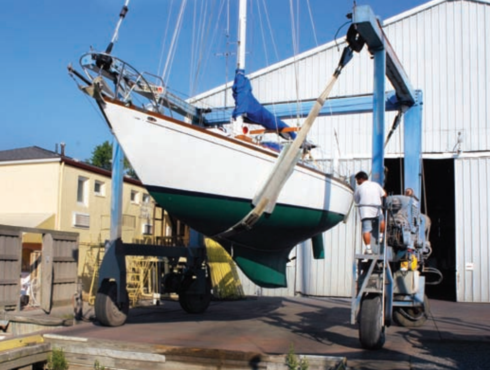
A skilled Travelift operator, like this one at Galesville boatyard (above), will be able to instinctively arrange rigging and place the slings, no matter the hull shape.
