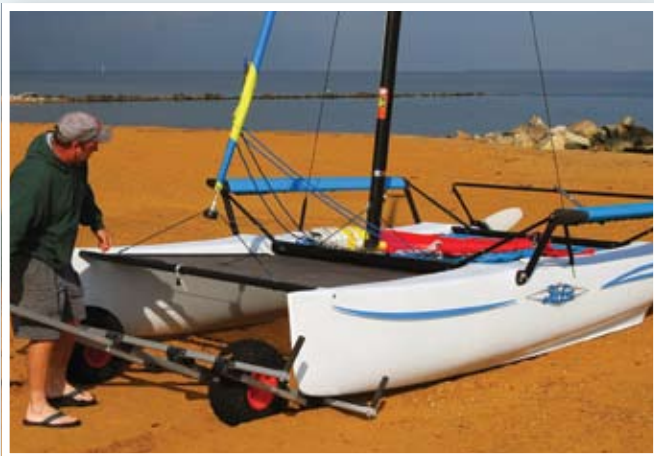
The heavy Hobie Getaway (left) favors durability over weight savings, while the Weta leans toward light, stiff panels.
