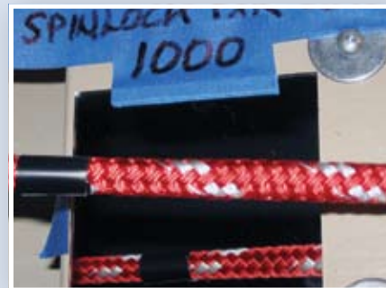
The neck is just ahead of the tape, and the fuzz is an inch or so ahead of the neck. The dark color on the underside of the line is in most cases from the trip bar. The dark mark on the top of the line is the point where the line pulls down into the cams.
