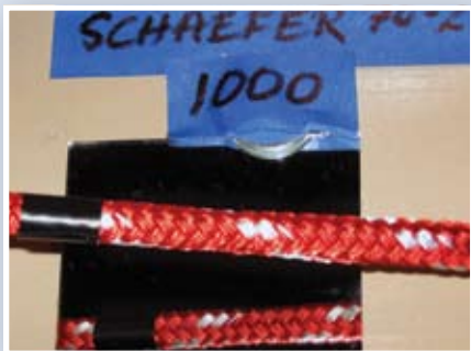
The neck is just ahead of the tape, and the fuzz is an inch or so ahead of the neck. The dark color on the underside of the line is in most cases from the trip bar. The dark mark on the top of the line is the point where the line pulls down into the cams.
