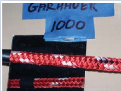
The neck is just ahead of the tape, and the fuzz is an inch or so ahead of the neck. The dark color on the underside of the line is in most cases from the trip bar. The dark mark on the top of the line is the point where the line pulls down into the cams.
